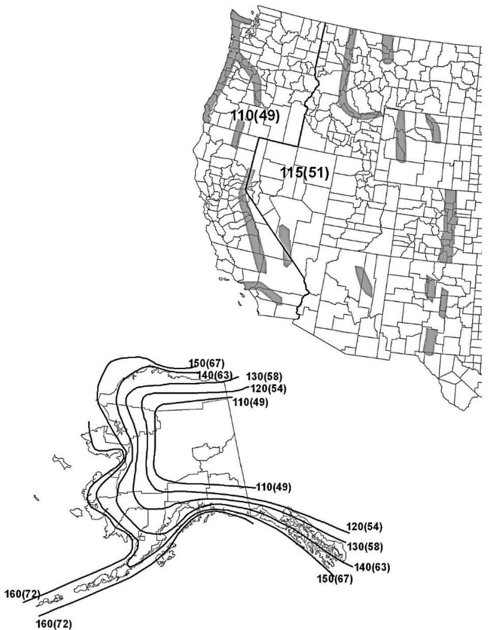
Figure 3.8-1a—700-Year MRI Basic Wind Speed, mph (m/s)—Western U.S. including Alaska (used with permission from ASCE)
